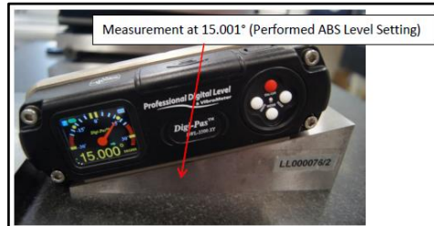
Figure 18 Measurement reading of DUT on 15.001° fixed angle jig
