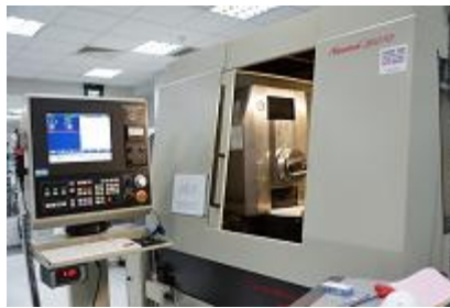
Figure 12 Nanotech® 350FG, Ultra-Precision 3-Axis Freeform® Generator
