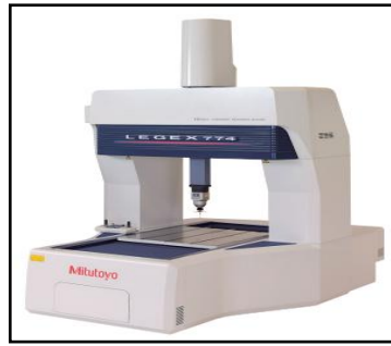
Figure 11 Coordinate Measuring Machine (CMM) Mitutoyo LEGEX Series [9]
